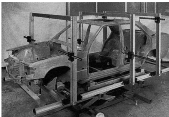
Figure 14.56 Autorobot measuring system used on the XLS II ( Kroll (UK) Ltd )
