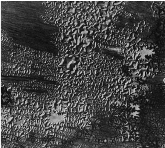
Figure 16.46 Wrinkling (Scott Bader Co. Ltd)
