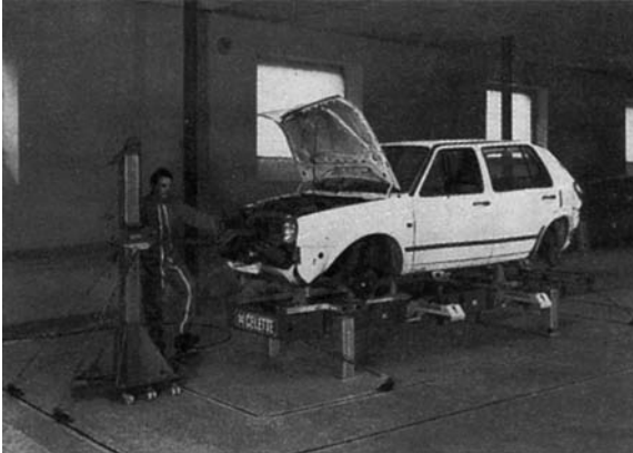
Figure 14.12 System 5000 pulling tower and frame (Celette UK)
