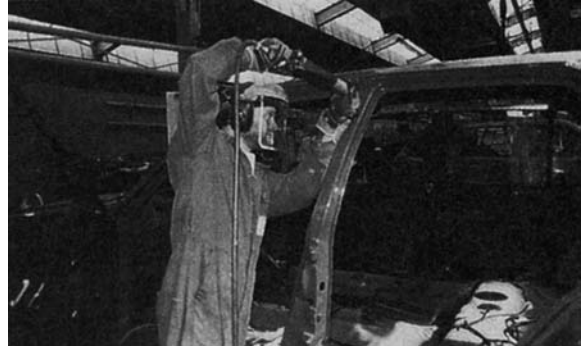
Figure 14.97 Cutting out damaged panels with a power saw ( Motor Insurance Repair Research Centre )
