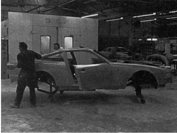
Figure 13.20 Panelled body shell sprayed in primer surfacer ( Aston Martin Lagonda Ltd )
