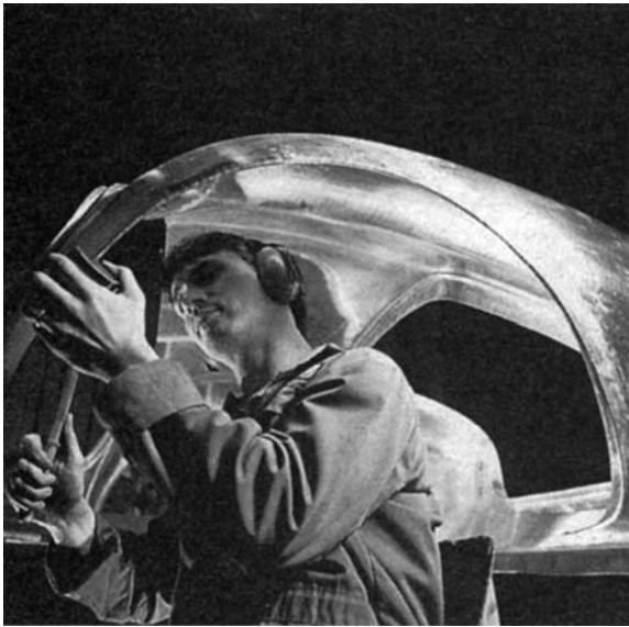
Figure 13.16 Planishing a hand-made panel ( Autokraft Ltd )
