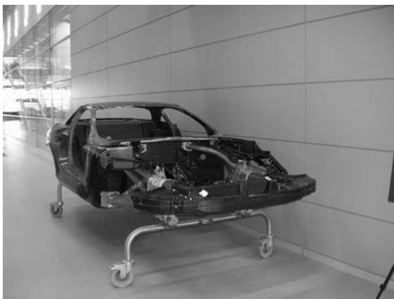
Figure 16.27 Mercedes Mchaven SLR body-in-white
