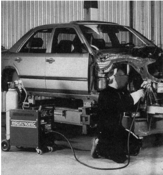
Figure 12.33 Application of MIG welding in body repair work ( Migatronik Welding Equipment Ltd )
