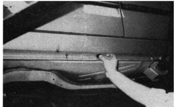
Figure 17.67 Sealing underbody ( Tuff Kote Dinol )
