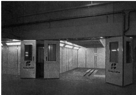
Figure 17.58 Corner installation showing two low-bake units, height 2.5 m (Spraybake Ltd)
