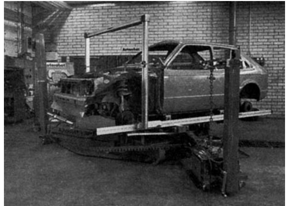
Figure 14.75 MacPherson strut measuring ( Kroll (UK) Ltd )
