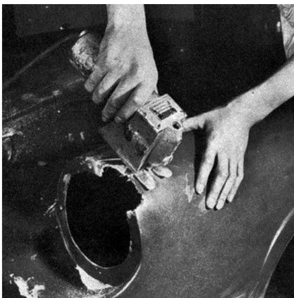
Figure 16.36 Removing damaged laminate
