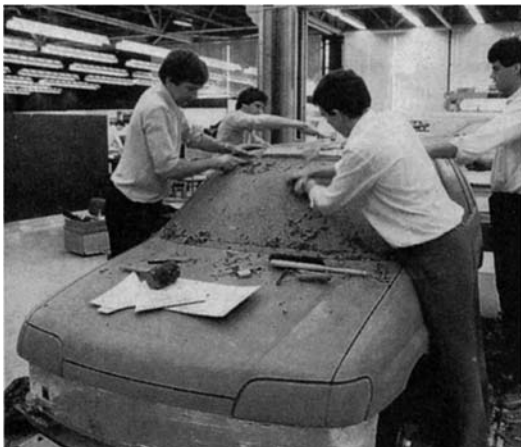
Figure 1.15 Full-size clay model ( Ford Motor Company Ltd )
