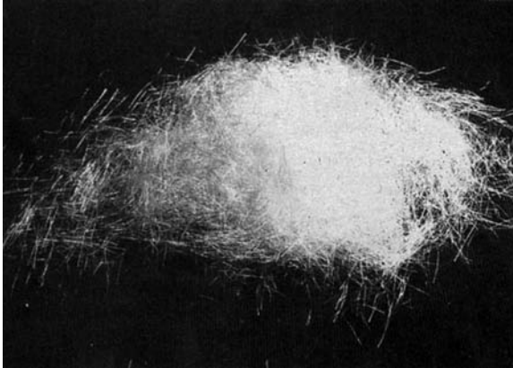
Figure 16.10 Chopped strands ( Owens-Corning Fiberglas )
