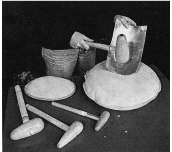
Figure 13.3 A panel being shaped by hollowing (Frost Auto Restoration Techniques Ltd)
