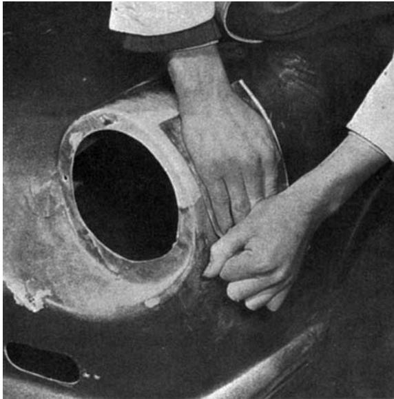
Figure 16.42 Finishing the laminate repair
