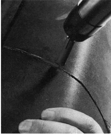
Figure 14.120 Tack welding split in bumper (Welwyn Tool Co. Ltd)
