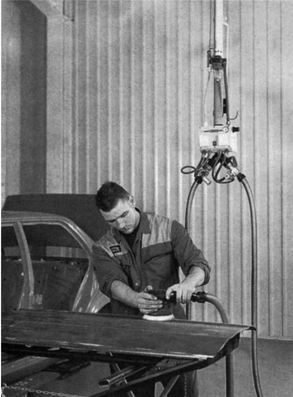
Figure 15.8 Central extraction unit ( Minden Industrial Ltd )
