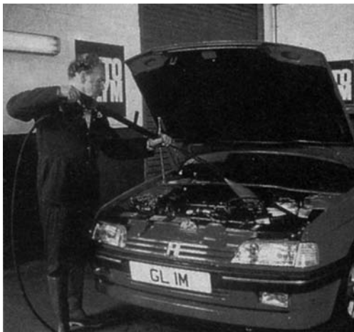
Figure 14.129 Pressure washing engine compartment ( Autoglym )
