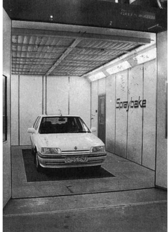
Figure 17.59 Interior shot of Green Booth designed to meet EPA regulations (Spraybake Ltd)
