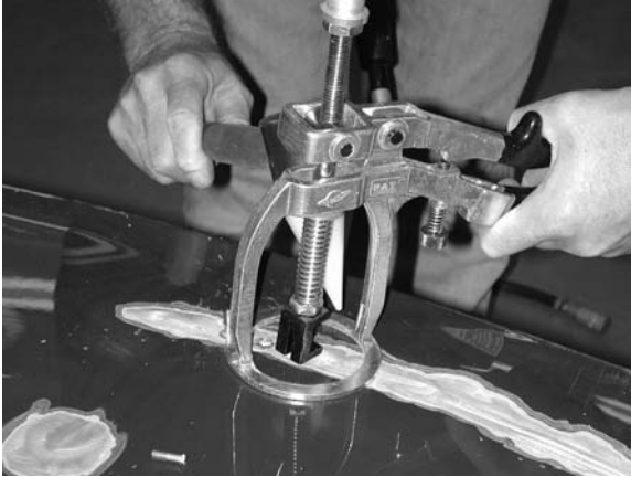
Figure 13.73 'MIRACLE' pulling tool (Courtesy of POWER-TEC®)
