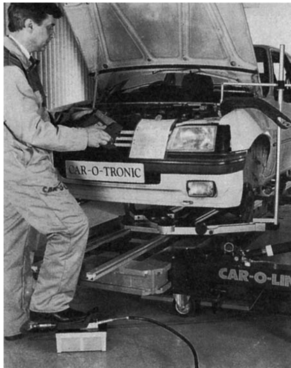
Figure 14.46 Pulling and measuring using the Car-O-Tronic ( Car-O-Liner (UK) Ltd )
