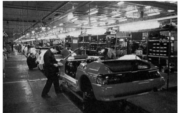
Figure 16.33 Vehicle undergoing interior trim ( Lotus Engineering )
