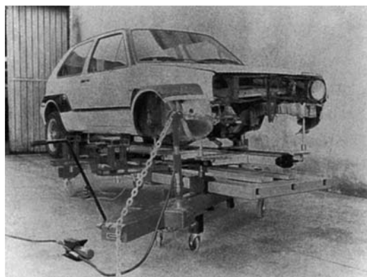
Figure 14.68 Alignment and repair using a measuring bridge system ( Blackhawk Automotive Ltd )
