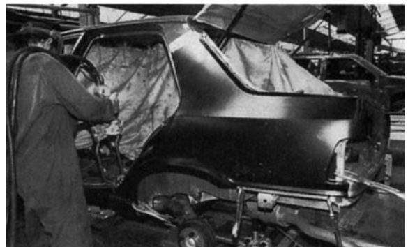
Figure 10.19 Pincer welding gun used in different locations in repair work ( Motor Insurance Repair Research Centre )
