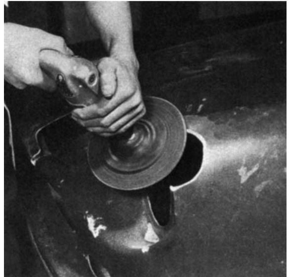
Figure 16.37 Scarfing the laminate
