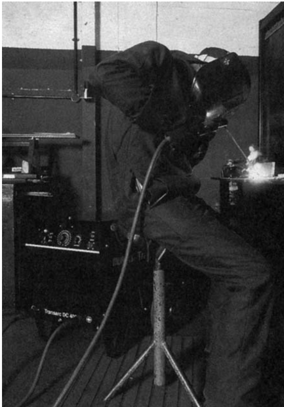
Figure 11.6 Welder wearing headshield and protective clothing ( Murex Welding Products Ltd )
