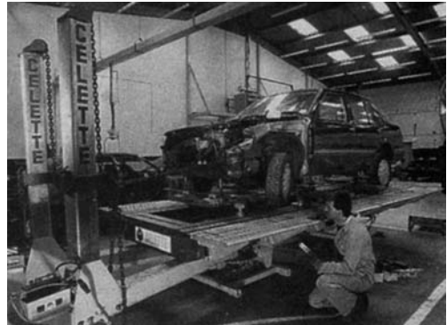
Figure 14.17 Bodymaster 2000 with Metro 2000 measurement system (Celette UK)
