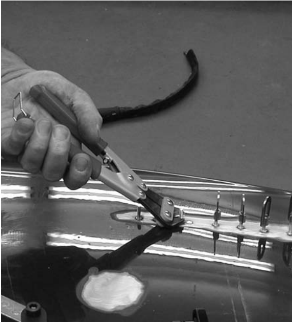
Figure 13.74 Snip-off the studs (Courtesy of POWER-TEC®)
