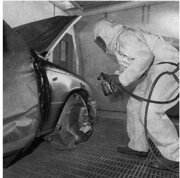
Figure 17.39 Spraying a vehicle wing ( DeVilbiss Automotive Refinishing Products )
