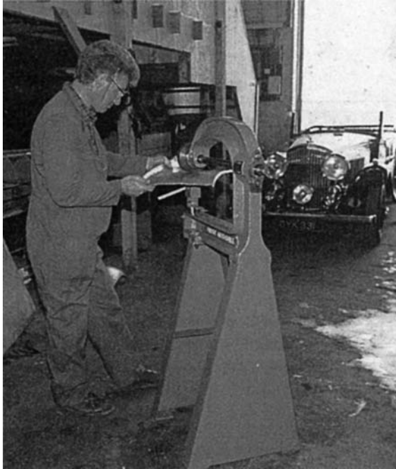
Figure 13.7 Wheeling a panel to restore a vintage vehicle ( Frost Auto Restoration Techniques Ltd )
