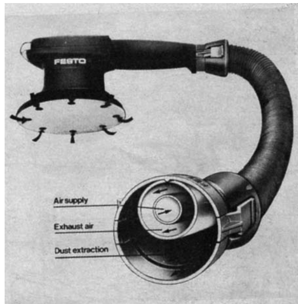
Figure 17.47 Festo random orbital sander ( Minden Industrial Ltd )
