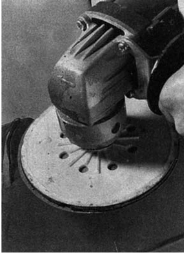
Figure 14.123 Weld dressing ( Welwyn Tool Co. Ltd )
