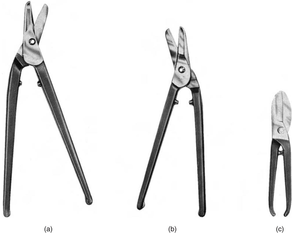
Figure 3.11 (a) Universal combination snips RH (b) universal combinations snips LH (c) standard pattern straight snips ( Sykes-Pickavant Ltd )
