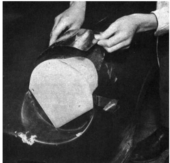
Figure 16.41 Removing temporary moulds
