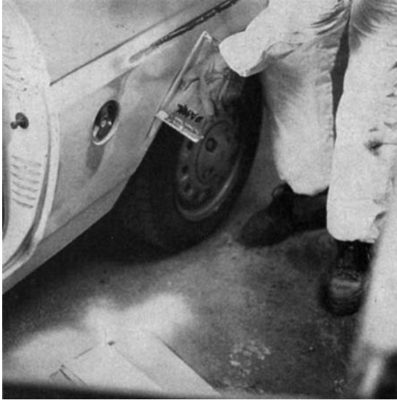
Figure 13.48 Shaping panel contour with abrasive paper and backing block ( Bondaglass-Voss Ltd )
