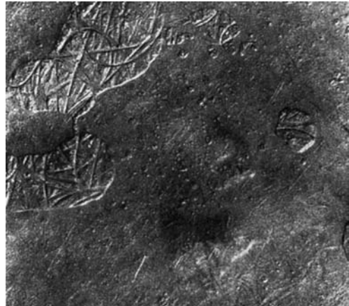
Figure 16.50 Severe blisters ( Scott Bader Co. Ltd )
