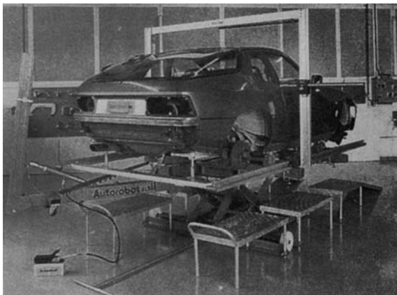
Figure 14.55 Autorobot XLS II system ( Kroll (UK) Ltd )
