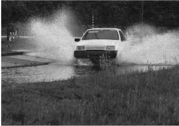
Figure 1.25 Water testing a prototype ( Ford Motor Company Ltd )
